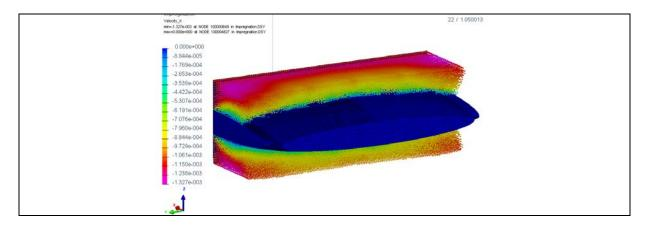
**Figure 3:** Impregnation of a plain weave unit cell at the meso level showing the velocity profile (*m*/*s*) during inflow with a constant velocity. A no-slip condition was used at the yarn interface surface and slip conditions at the other surface.
