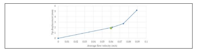
**Figure 2:** *Experimental and modelling results. The graph shows the average flow velocity (m/s) versus the tip displacement of the rubber rod (mm). The blue line represents the experiments, the green dot the simulation results.*
