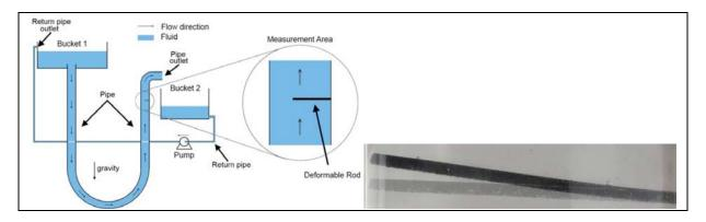
**Figure 1:** Experimental set-up to measure the flow induced deformation of a rubber rod. The left hand side shows the schematic setup of the experiment while the right hand side shows the detail of the rod in the pipe during the experiment. The deformed (black) and undeformed (grey) shape are shown in the photograph.
